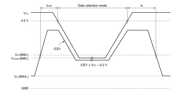
RemarkOn the data retention mode by controlling /CE1, the input level of CE2 must be  $CE2 \ge Vcc - 0.2$  V or $CE2 \le 0.2$  V. The other pins (Address, I/O, /WE) can be in high impedance state.
